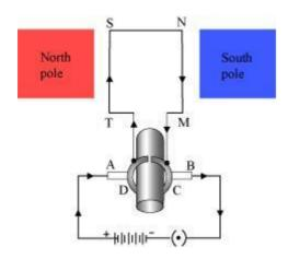
The current flows through the coil in the direction TSNM. The reversal of current through the coil MNST repeats after each half rotation. As a result, the coil rotates unidirectional. The split rings help to reverse the direction of current in the circuit. These are called the commutator.
