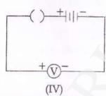
In which of the circuits, the voltmeter/ammeter is likely to be damaged, on plugging the key? (a) I (b) II (c) III (d) IV
