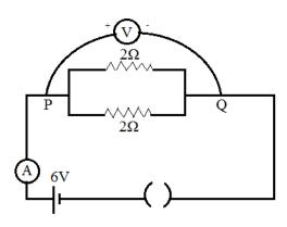
Reena measured reading of voltmeter 'V' which gives potential differences between P and Q she should find the reading to be: (a) 2 V (b) 4 V (c) 6 V (d) 8 V
