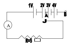
Ans. when J is connected to A I=V/R=3/5A=O.6A When J is connected to B V=1+2+3+4=10V I=10/5=2A
