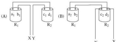
Student A connects the terminals marked  $b_1$  and  $c_1$  while B connects the terminals marked  $d_2$  and  $c_2$  in their respective circuits at the points marked X and Y.
